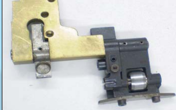
Lower Side Guide Ass'y AKA: Bearing Drive Side #53.072.203
