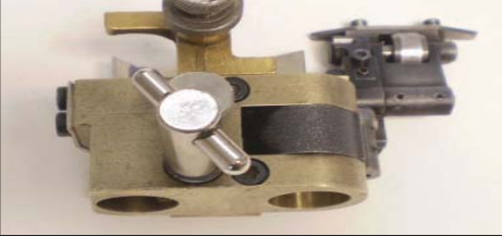
Side Guide Ass'y - Operator Side A.K.A: Bearing O.S. #53.072.204
