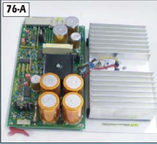
76-A NTK-85 Power Supply Board #81.186.5155
