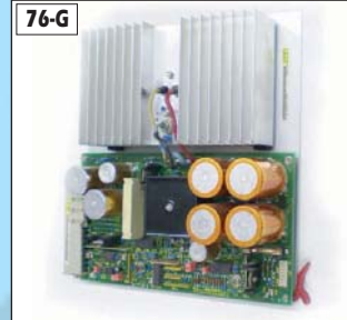
76-G NTK-85 Power Supply Board #81.186.5155
